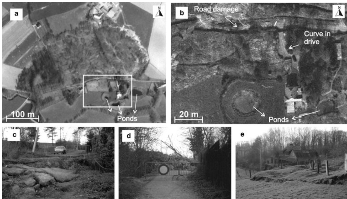
Figure 6 The Hekkebrugstraat landslide: (a) aerial photograph (NGI, 1996). White rectangle indicates enlarged area of De Saedeleer's garden (DS in Figure 4b,c) shown in (b); (b) detail of orthophoto (OC-GIS Vlaanderen, 1998) showing part of De Saedeleer's garden. In the north the road is damaged by debris. The curve in the drive is caused by the downslope movement of the debris. This movement occurred after April 1996, because the curve is not present on (a); (c) damage to the road and electricity lines (2001). In the back, the 8-m-high main scarp can be distinguished; (d) the downward movement of the debris blocked the road (2001); (e) since 1999, the landslide foot has been located only a few metres from De Bo's house (DB in Figure 4b,c).
